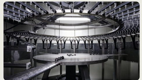
Top: Airflow analysis in our wind tunnel Bottom: Our in-house rain erosion test rig
